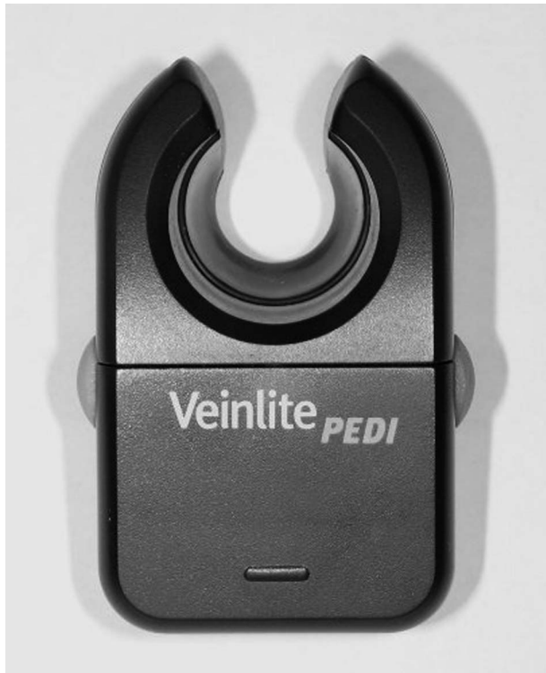
FIGURE 1. Veinlite PEDI Transilluminator Vein Finder ( http://www.veinlite.com ).
